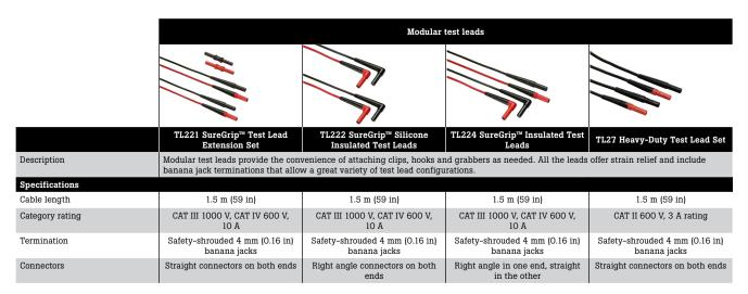
This wide variety of clips and probes allows you to configure the modular test leads to individual needs. Use with modular clips (Table A) or modular test probes (Table B).
